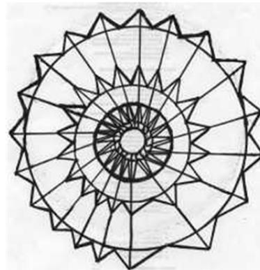
**Figure 8B.** Overlay of Three Layers of Twenty Sensors
