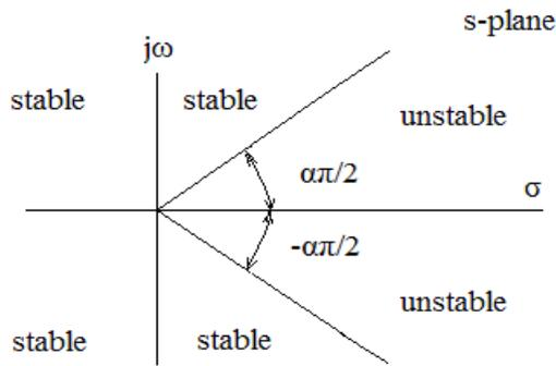
Figure 1. Stability region of linear fractional-order system with  $\alpha$
