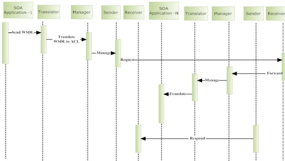
**Figure 13.** AUML Sequence Diagram for the Agent-based MOM
