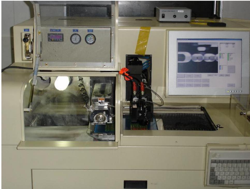
**Figure 10.** Photo of automatic wafer dicing
